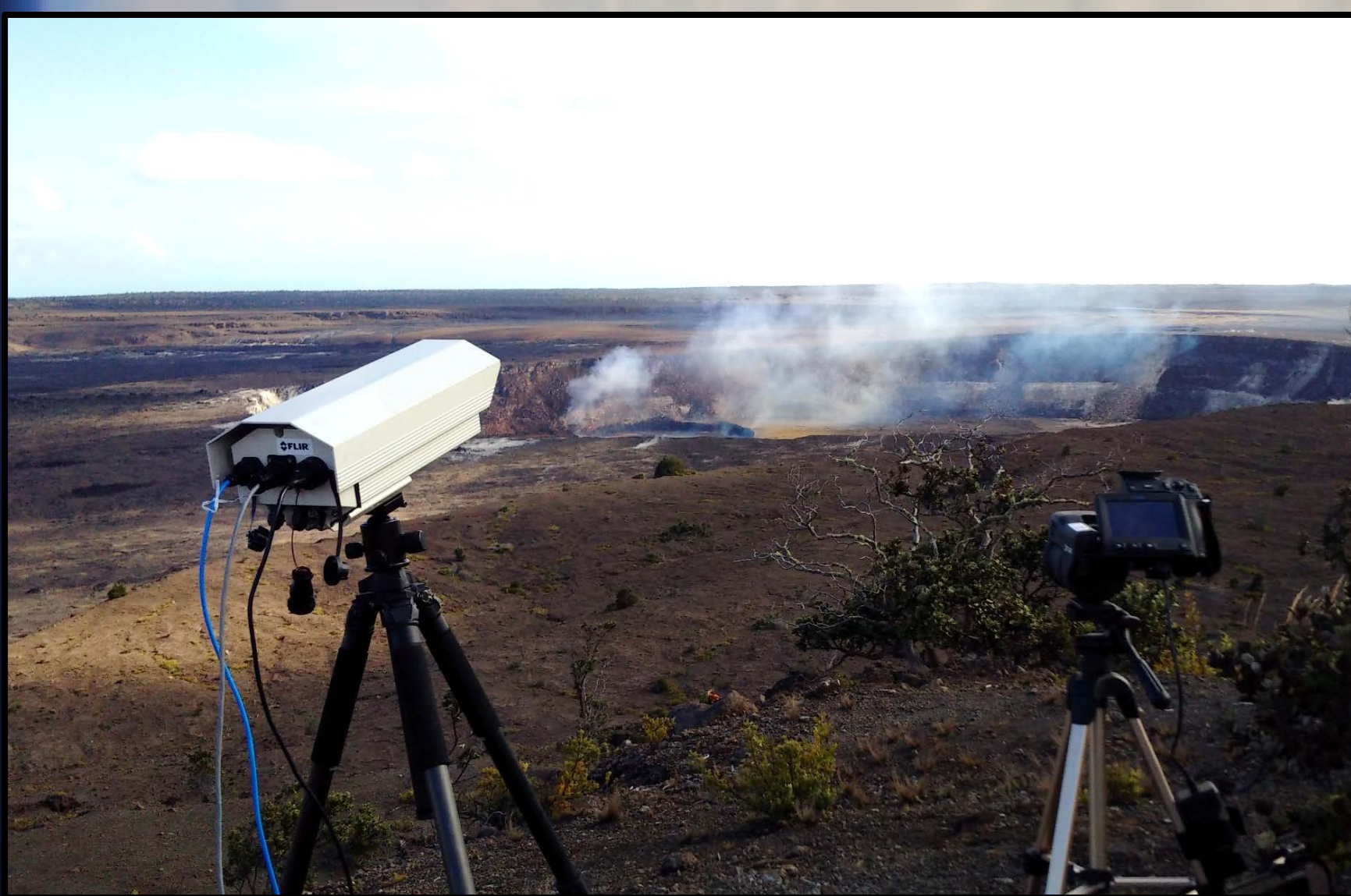
Figure 1: Field image of the new miniature multispectral TIR camera (MMT-Cam) deployed at Kilauea caldera in January, 2017. The camera is capable of acquiring up to 6 wavelength channels at 7 Hz in the 8 – 12 μm region.
