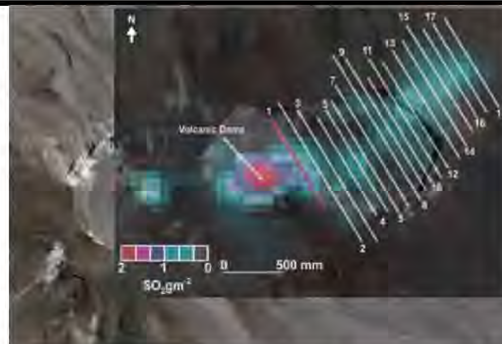
ASTER-based retrieval of the smallest recorded passive SO 2 plume from Lascar Volcano, Chile (from Henney et al., 2012). Detection of such small, low gas flux plumes is only possible with high-spatial, high-SNR, multispectral TIR data, which would be routine with I-THEMIS.
