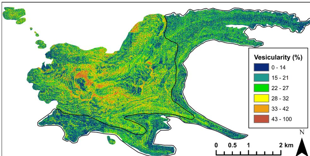
Figure 4: Vesicularity result for the BGMF, produced using a linear deconvolution model on the MASTER emissivity data and the two end-members (figure 2). The degree of vesicularity varies from 0 to 81%, with variation between individual flows and within a flow being up to 80% and 25%, respectively.
