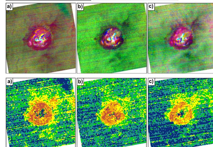
Figure 6: ASTER DCS of the Chaitén dome using bands 14 (11.32 μm), 12 (9.10 μm), and 10 (8.29 μm) in R, G, B, respectively. a) 12/31/10. b) 04/06/11. c) 02/13/12.
