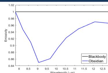
Figure 2: End-member emissivity spectra used in the linear deconvolution model.
