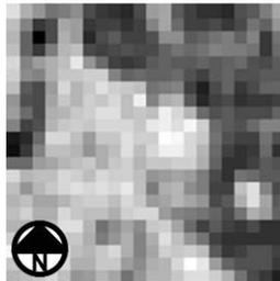
**Figure 2.** Comparison of the spatial resolution for each of the three ASTER subsystems over a 2 km portion of São Paulo, Brazil. The ASTER L1B scene was acquired on 19 March 2002 (13:23:17 UT). All images have a 2% linear stretch applied. (top) 15 m/pixel VNIR band #2 (0.63-0.69  $\mu\text{m}$ ). (middle) 30 m/pixel SWIR band #7 (2.24-2.29  $\mu\text{m}$ ). (bottom) 90 m/pixel TIR bands #12 (8.93-9.28  $\mu\text{m}$ ).
