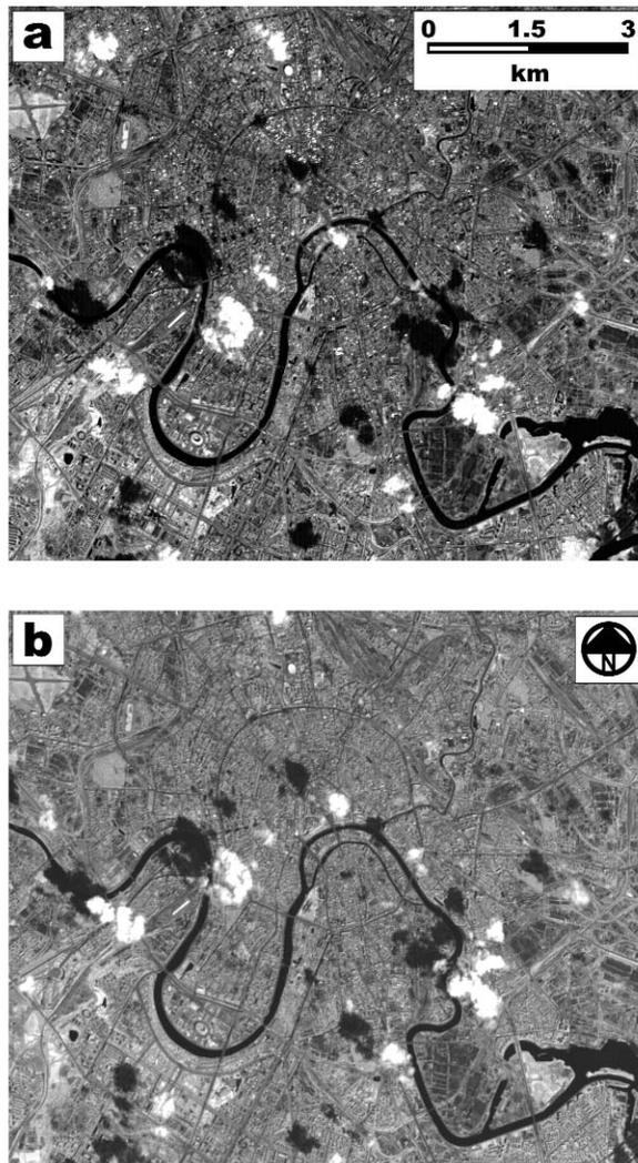
**Figure 3.** Band #3 (0.76-0.86  $\mu\text{m}$ ) ASTER L1A gray-scale images of Moscow, Russia collected on 28 August 2000. (a) Band #3n (nadir-looking telescope). (b) Band #3b (back-looking telescope). Band #3b is acquired with a different viewing geometry (note the cloud positions in each image with respect to their shadows). Images pairs such as this provide the ability to generate along-track digital elevation models (DEMs).
