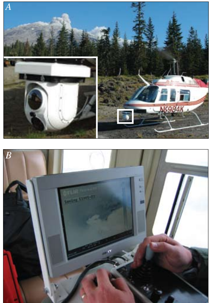
Figure 1. Forward Looking Infrared (FLIR) thermal and visual video imaging system used during airborne observations of Mount St. Helens, 2004–2007. A , FLIR instrument mounted on nose of Bell 206-L helicopter. Inset shows infrared (top) and visual video (bottom) lenses. B , Remote control panel used to display infrared and visual video streams, to control orientation of sensors using a joystick, and to capture data.
